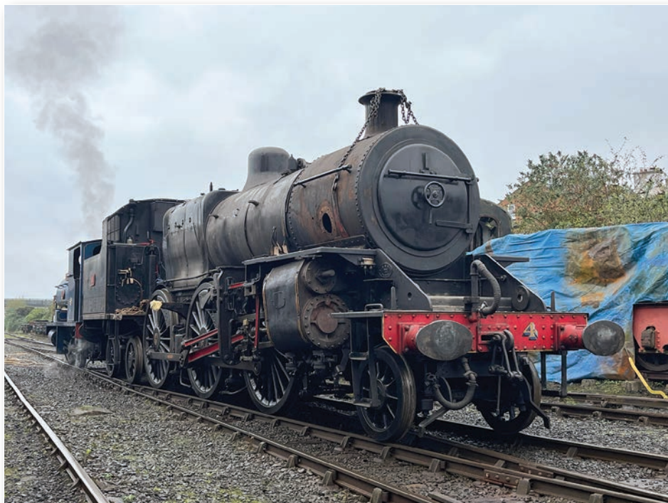
No.4 vaguely resembles a Mogul as she is shunted by 3BG towards the sheer legs for boiler removal on 2nd November. (Photo: D Tartaglia)
