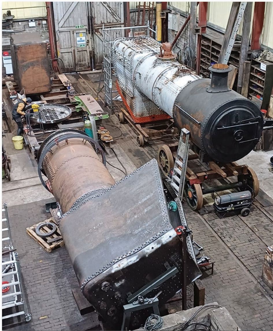
Two “NCC” boilers in the Dunleath workshop on 2nd February 2025. On the left, on the rotator, is the mogul boiler complete with several rows of nice new rivets, added during the Christmas break. Directly beyond it, the front tubeplate is being worked on. Directly beyond that again, the copper inner firebox may be seen. No.4’s boiler, with dome-cover removed revealing the periscope-like regulator valve, is on trolleys on the right: just at a very useful time to provide cross-referencing. (Photo: PA Scott)
