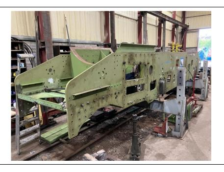
As of mid-2025, the Mogul frames are seen in the Dunleath Workshop. The saddle and stretchers are in position. Riveting of the frames is to commence soon. Both the Mogul and the later 'Jeeps' (like RPSI No.4) were based on the LMS 2300 class tank engines, which provided the design of the working parts and boiler.
